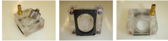
Figure 3. Water path wedges manufactured by Olympus® (4)
